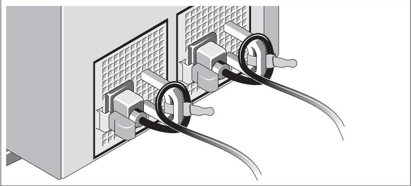
Attach the power cord retention bracket on the right bend of the power supply handle. Bend the system power cable into a loop as shown in the illustration and attach to the bracket's cable clasp.
